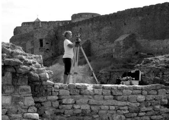
Iryna Karashevych surveying the shore ward with a total station. Above are the walls of the garrison ward and to the left the top of the citadel
